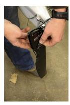
• **S14 & S14-LV RUDDER UPGRADE:** When adding an over stern rudder to the S14 and S14-LV, you will need to purchase the Hybridfoil Rudder and 7meters of 1.7mm Dyneema steering line. The boat already comes fitted with the rudder post tubing, steering line tubing and the steering toe pedals for a convenient upgrade. Follow the instructions above to install the Hybridfoil Rudder into your boat, along with the retraction line, which is included in the spare parts bag.
