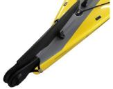
Put plastic fender washer on rudder post before installing – turn rudder clockwise to the bow to install
