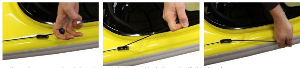
Pull Up, then Forward and then down to deploy and lock the Hybridfoil rudder for use.
