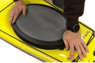
Line up the centerline and work around from one end to the other and check the complete edge is down
