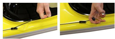
Pull up and then back to deploy the Compact rudder.
