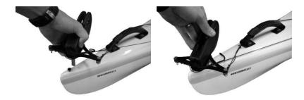
• For removing the rudder blade from the steering housing, you want the rudder to be retracted on the deck. Simply remove the pin from the side of the rudder and then pull out the locking plug. Then pull the knot from the rudder blade to complete removal.
