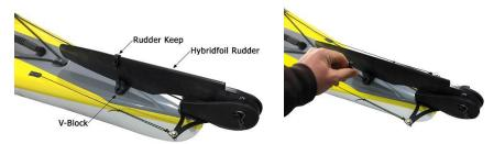
• To deploy the rudder, make sure to release the bungie hook from the rudder blade at the V-block and then lift up and pull forward the end of the rudder line by your right hip. Once the blade is fully deployed, push the line back down to cleat it off. To stow the rudder, simply lift up on the rudder line and move the toggle back to the cleat, whereby the spring in the rudder housing will rotate the rudder blade onto the deck.
