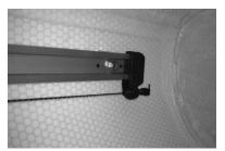
At this point, move back to the rudder and in the spare parts bag you will find 2 small metal posts, round wire cotter pins and rope guide. Push the pin through the rope guides on each side of the rudder yoke and then put the wire cotter pins in the bottom of the posts to secure them. Run the steering line around the rope guide and with a helper, tie them off with the steering pedals evenly at around 15 degrees of forward tilt and the rudder straight.
