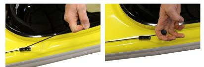
Pull up and then back to deploy the race rudder.
