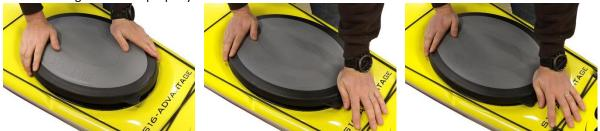
Line up the centerline and work around from one end to the other and check the complete edge is down
