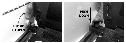
To operate the Quick Release footbrace, you need to open the 2 upper plastic cams and then the lower central aluminum cam along the keel. When you open the plastic cams, you need to flip 180 degrees and then press down on the top firmly. This will help disengage the teeth on the cam bolts from the teeth in the plastic tracks.
