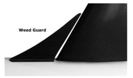
• The weed guard should be placed 2 mm in front of the rudder for adequate protection. We recommend using a
