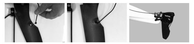
• **Rudder Alignment:** When changing the angle of your foot pedals or installing new steering line, make sure to check the alignment of your rudder. Ideally, a helper can hold the rudder straight, while you tighten the steering line forward of the foot-pedals while making sure both pedals are at the same angle.
