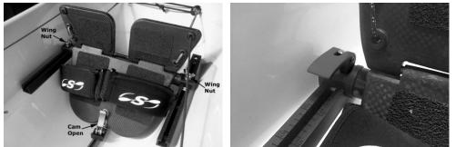
Starting in 2012, the top tube-end fittings are fastened with plastic cams
